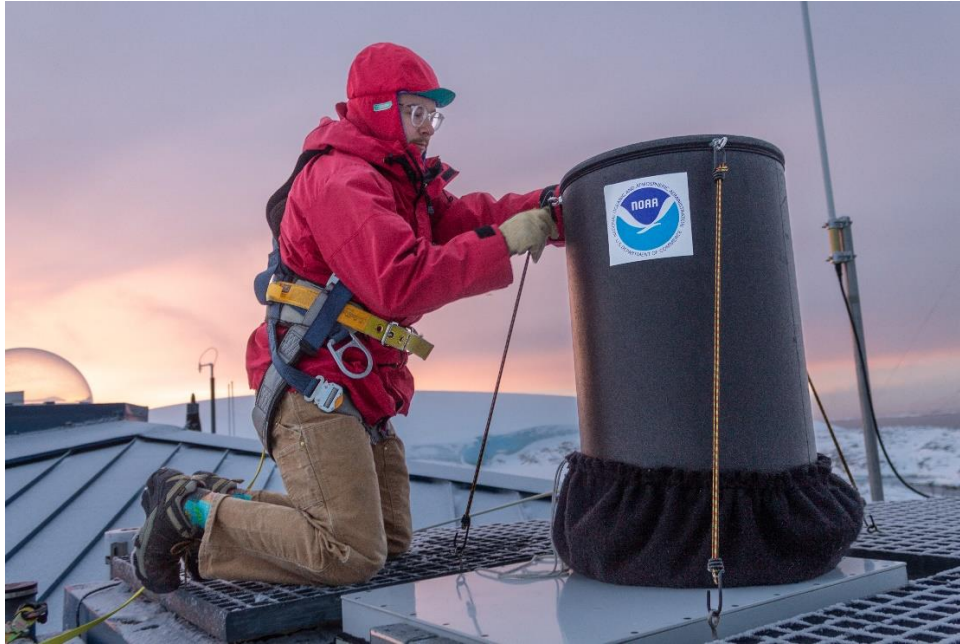
Research Associate performs an SUV Absolute Calibration (O-264-P) on the Terra Lab roof.
